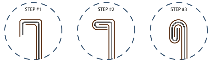
Twin-Loc Seaming Operation
